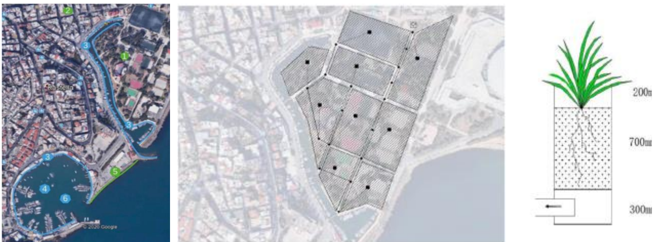
Figure 43. Drainage area analysed by SWMM Model of the Akti Dilaveri's left bank and biofilter columns
